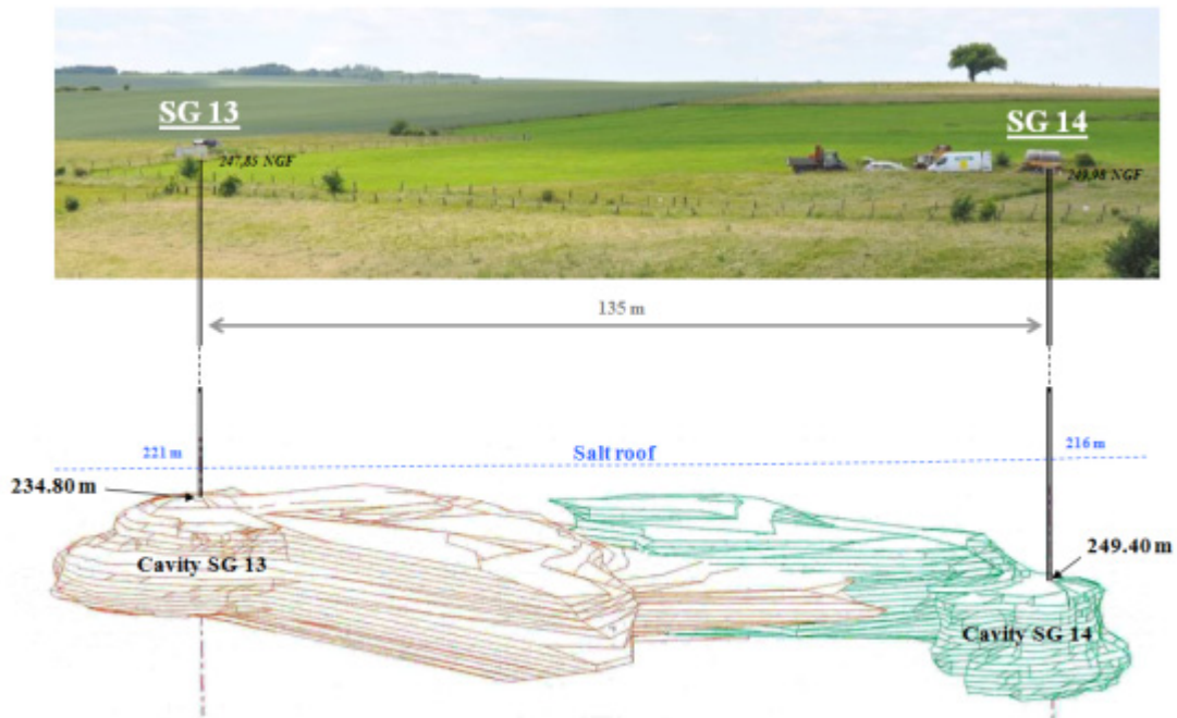
Figure 1 - 3D view of the SG13-SG14 cavern (From November 2000 sonar survey; the cavern is viewed from East to West with a 10° downward dip angle).
